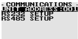
Enter the communication address of the instrument. If more than one instrument is connected via a multidrop network then the address of each instrument must be unique. A unique address allows commands to be sent to an individual instrument as well as it also prevents all the instruments on the bus replying simultaneously.
