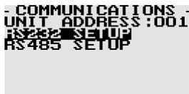
The ASCII out protocol address range is 0 to 255. The Modbus address range is 001 to 247.
