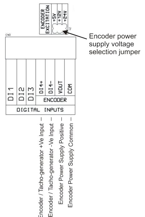
**Encoder with NPN (Open Collector) or Totem-Pole (Push Pull) output**
