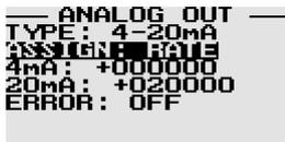
Select the source for the analog retransmission. The source can be selected from the “WEIGHT”, “RATE”, “TOTAL 1”, “TOTAL 2” or “SPEED”.
