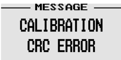
Calibration constants CRC error. The instrument could possibly have a non-volatile memory failure in which case the instrument will then have to be returned to the factory.
