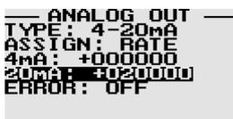
Enter the display value that corresponds to the selected analog output high value. E.G. 20.000 display counts = 20mA. (4-20mA analog output type shown).
