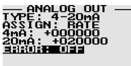
Enter what must happen to the analog output when an error occurs with the measured weight. eg. Over-range, Under-Range etc. The analog error can be set to:
