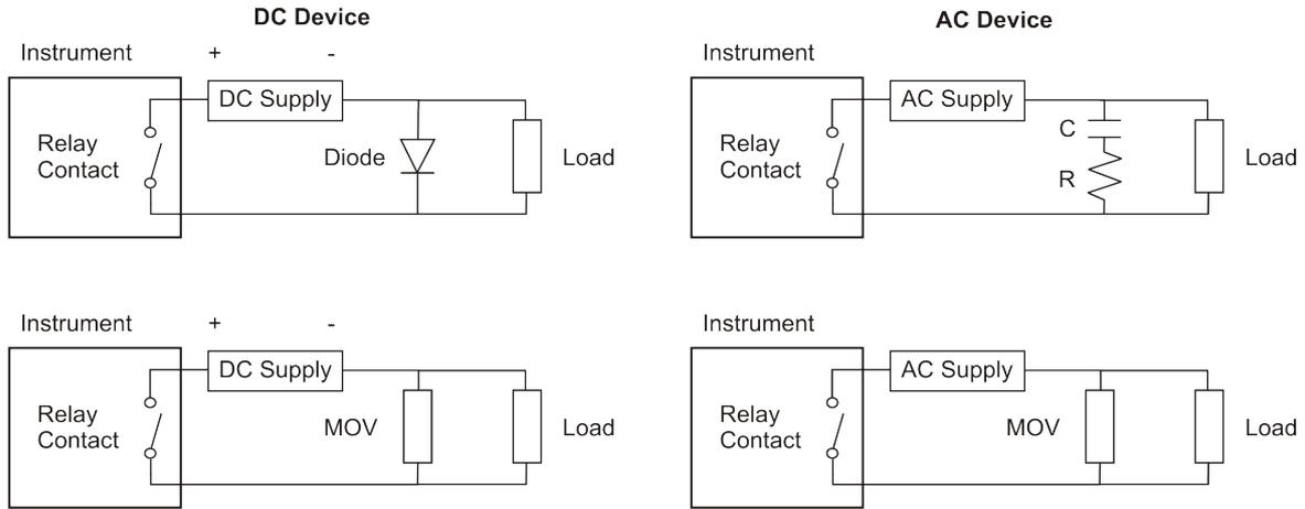
An optional noise suppression device can be ordered. Install these devices as close to the load as possible.
