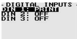
This menu option is only shown if either the RS232 or RS485 ASCII Out mode is selected. This digital input allows the user to print the display value via the RS232 or the RS485 interface. The print LED will briefly illuminate when the digital input is activated.
