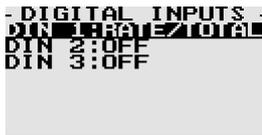
The digital input will toggle the LED display between showing the rate and the totaliser 1 value. The rate LED will illuminate to indicate that the LED display is showing the rate value alternatively the total LED will illuminate to indicate that the display is showing the totaliser 1 value.
