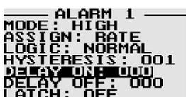
Enter the alarm on delay value in seconds that the alarm condition must persist before the alarm is activated.
