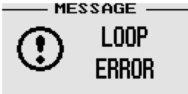
The LCD display will briefly flash the loop error message every 5 seconds to indicate that a mA loop error has occurred. This error message will only be shown if the analog out has been set for any of the mA ranges.
