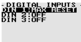
The digital input will reset the maximum recorder rate, speed and weight values to the current values.
