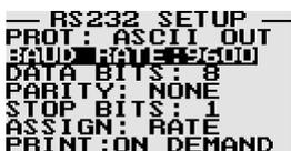
Select the communication baud rate. The baud rate can be selected from “1200”, “2400”, “4800”, “9600”, “19200”, “38400”, “57600” and “115200” baud.
