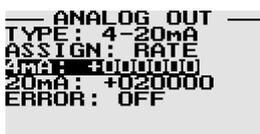
Enter the display value that corresponds to the selected analog output low value. E.G. 0.000 display counts = 4mA. (4-20mA analog output type shown).
