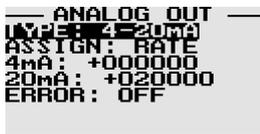
Select the analog output type. The analog output type can be selected from “OFF”, “0-20mA”, “4-20mA” or “0-10V”.
