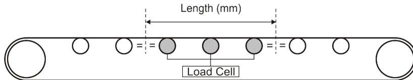
**Complete conveyor on load cells**
