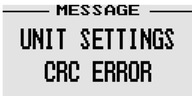
Unit settings CRC error. Load default settings to restore to factory defaults. If the error message still persists then it could possibly be a non-volatile memory failure in which case the instrument will then have to be returned to the factory.
