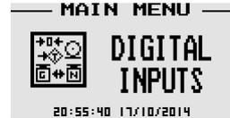
This menu configures the three digital inputs. The digital inputs can be configured for specific functions as listed below.
