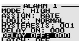
Enter the alarm off delay value in seconds that the alarm condition must persist before the alarm is de-activated.
