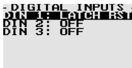
The digital input will reset any of the latched alarms when the alarm condition has been removed. This menu option is only displayed if any of the alarm latch functions have been enabled.
